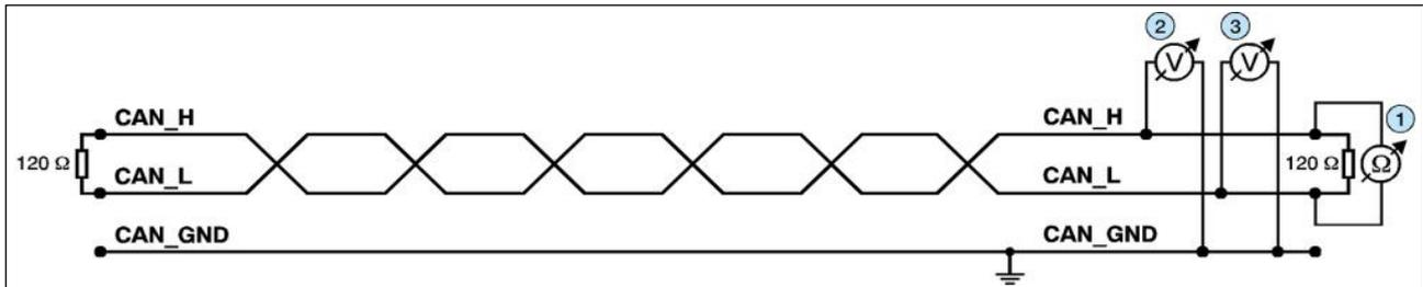
Figure 10: Simplified diagram of a CAN network
