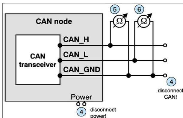
Figure 12: Measuring the internal resistance of CAN transceivers
