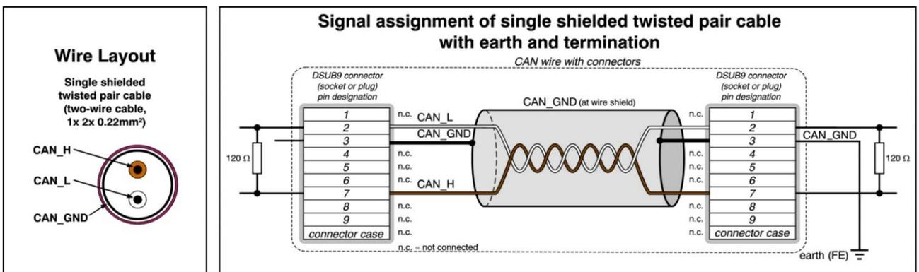
Figure 6: CAN wiring for light industrial environment
