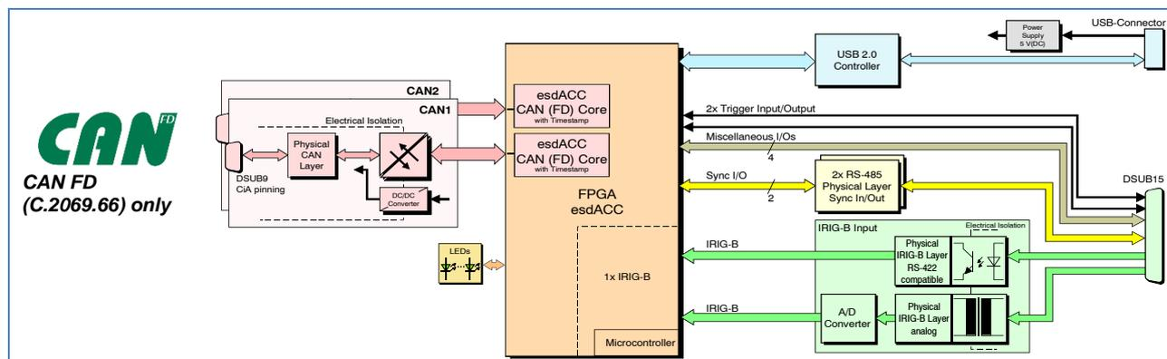
Figure 2: Block circuit diagram of CAN-USB/400(-FD)-IRIG-B
