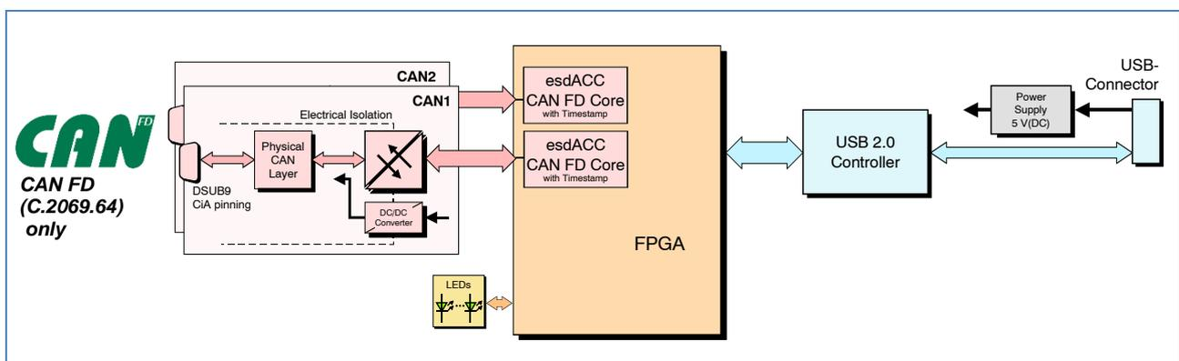
Figure 1: Block circuit diagram of CAN-USB/400(-FD)
