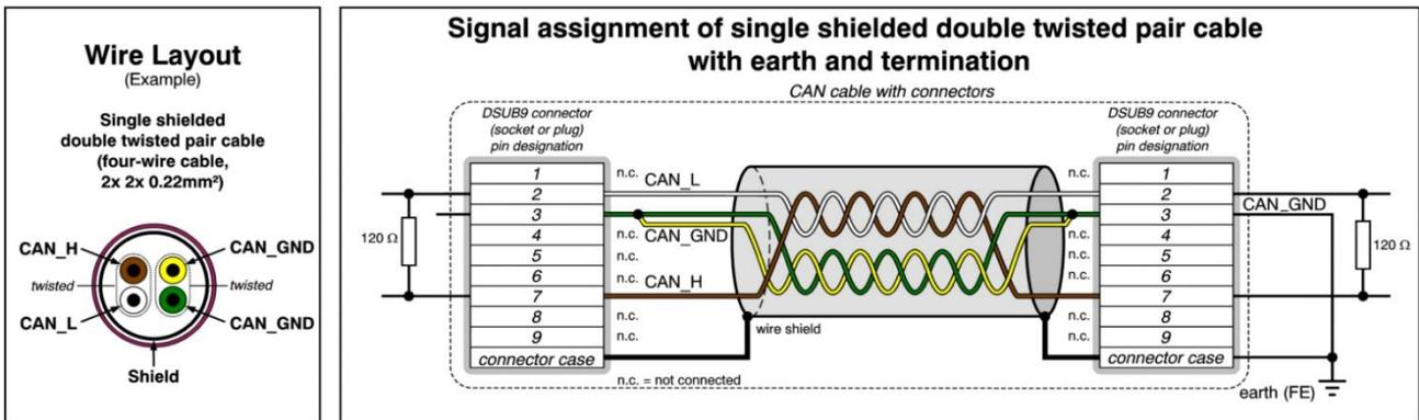
Figure 8: CAN wiring for heavy industrial environment
