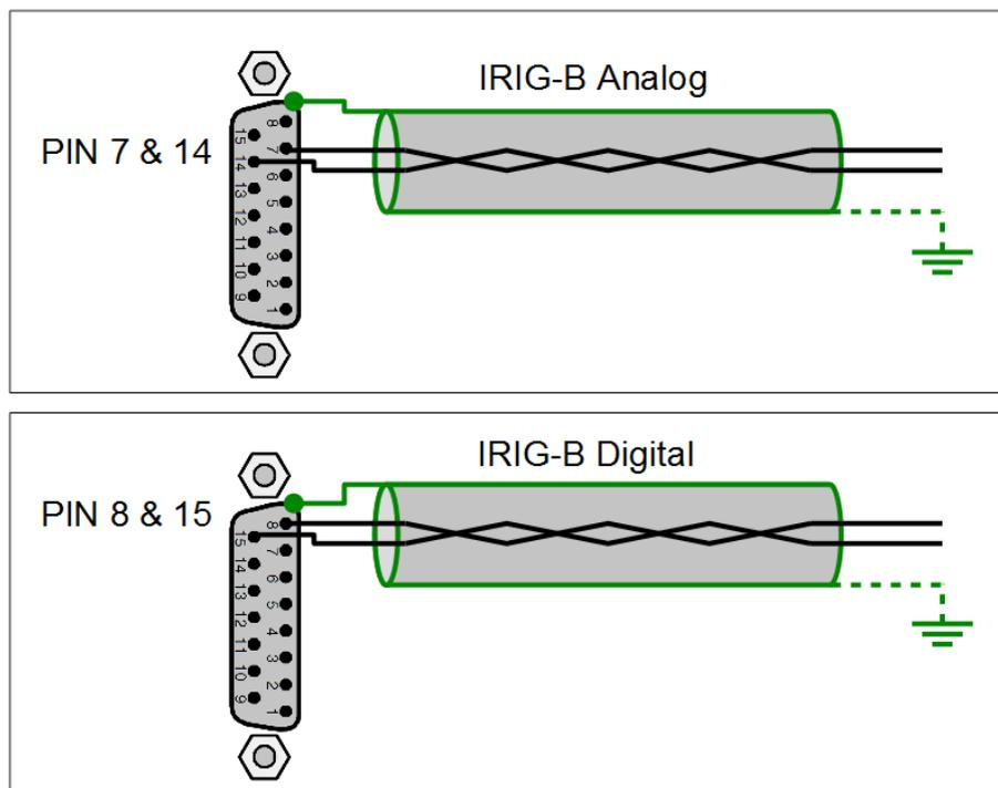
Figure 5: IRIG-B wiring guidelines
