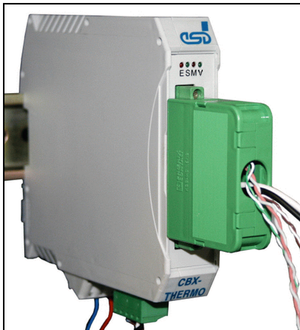
Fig. 4: Connection with cable housing to improve cold junction compensation
