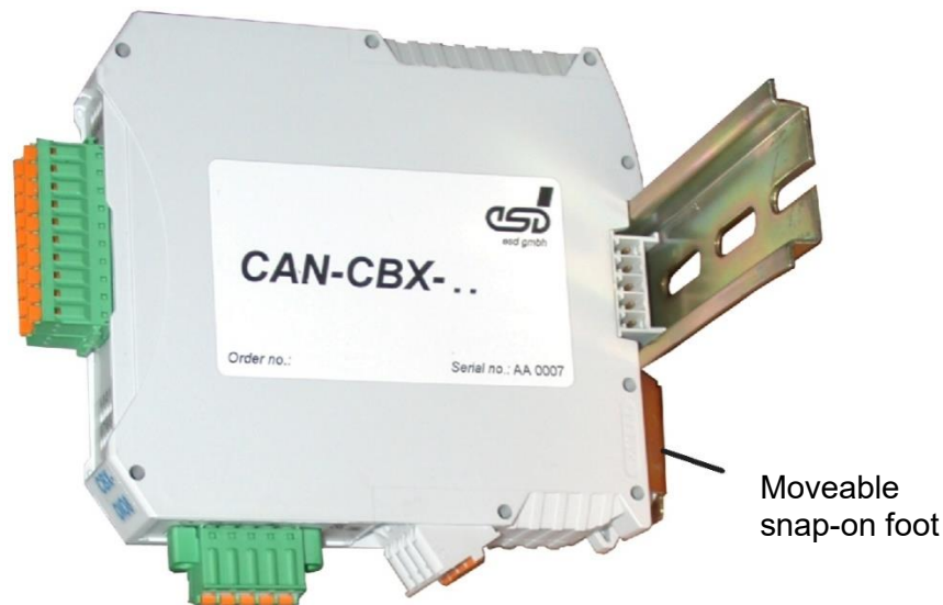
Figure 18: Mounted CAN-CBX module
